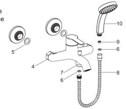
**NOTE:** When tighten the nuts, use strap wrench or soft cloth between product and regular wrench to protect the finish.
